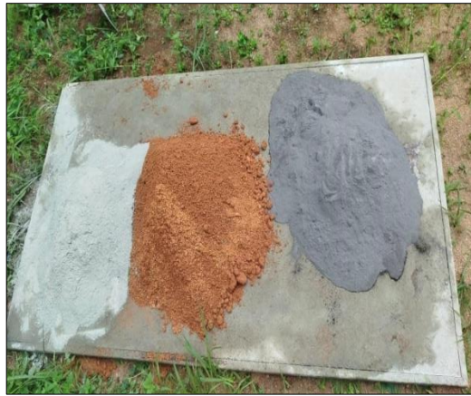
Figure 2 Batching done for the OPC, Fine Aggregate and the Coal Ash (Note: The Coal Ash has already been mixed with the Calcium Chloride)
