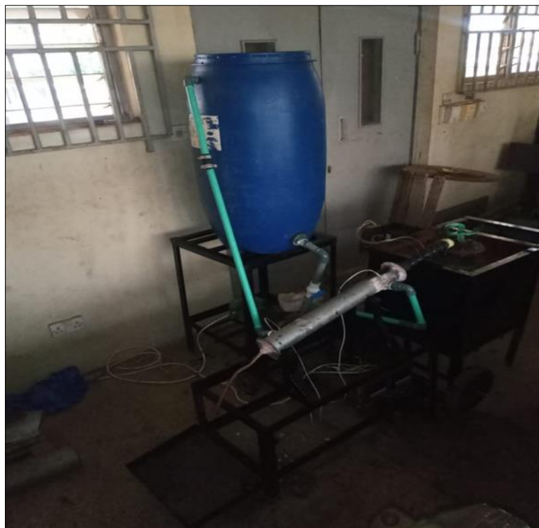
Figure 2 The three units of the pyrolysis plant
