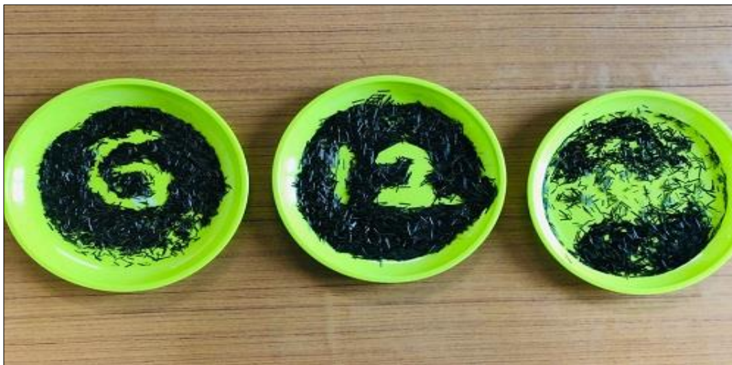
Figure 1 Chopped Basalt Fibre of 6 mm and 12 mm Length
