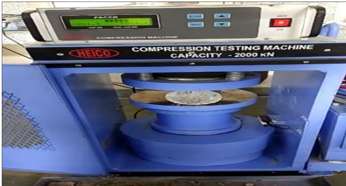
Figure 3 Split Tensile Strength Test Set-Up
